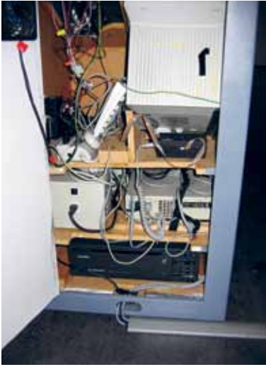
Open console of the installation Karlsruhe Moviemap (version 1991) The components originally used are easily identifiable: the Apple Macintosh Portrait Display (above), the Apple Macintosh IIsi and the Pioneer laser disc player LD-V8000 by (below). Photo © ZKM | Karlsruhe
